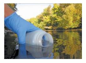
Water sample is collected at the waterbody being sampled and brought back to lab
